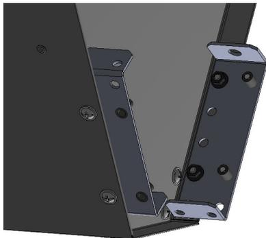
Installation of connector at the back of the curtains
