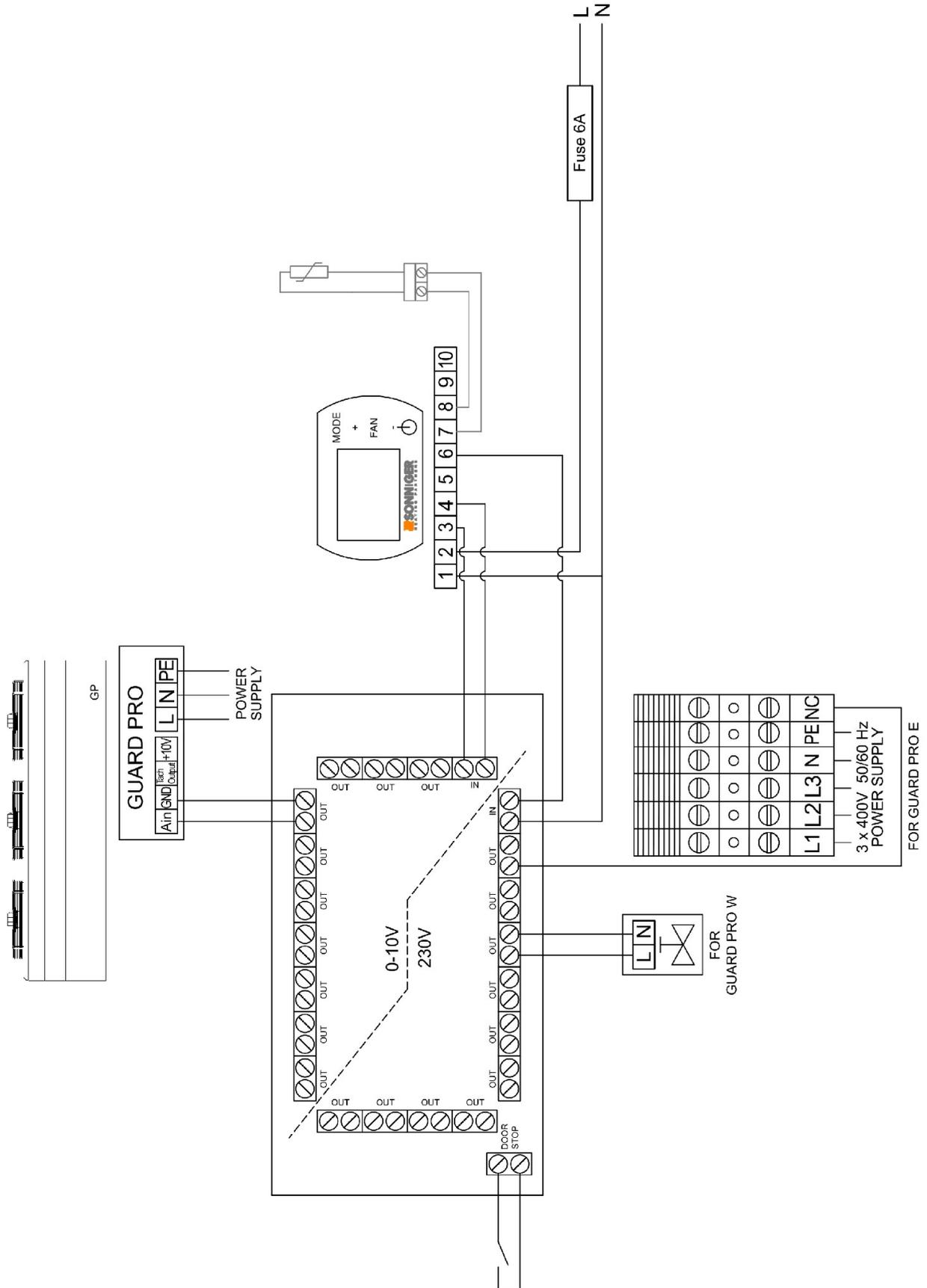
The Multi 10 EC control box allows to connect and control up to 10 GUARD PRO and 10 servomotors. The control of the unit motors is via INTELLIGENT WIFI EC, there is a possibility to connect DOORSTOP switch to it. The thermostat has a primary function when connected to the unit with the Doorswitch.
